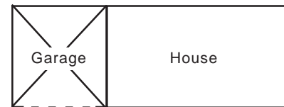
Figure 26 - If the wall of the main house is in line with the wall containing the door of a garage with a room over it, the adjoining wall may help brace the garage.
